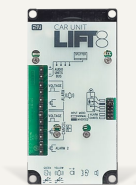
2N® Lift8 MACHINE ROOM PCB
